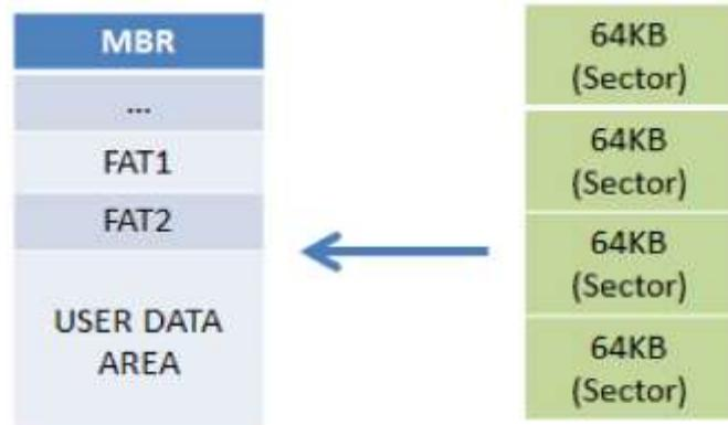
Heading address of user data area shall match with the heading of 64KB boundary of SD logical address.
